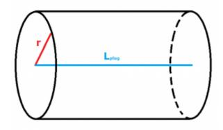
where r is the inside radius and  $L_{plug}$  is the length of the plug.
